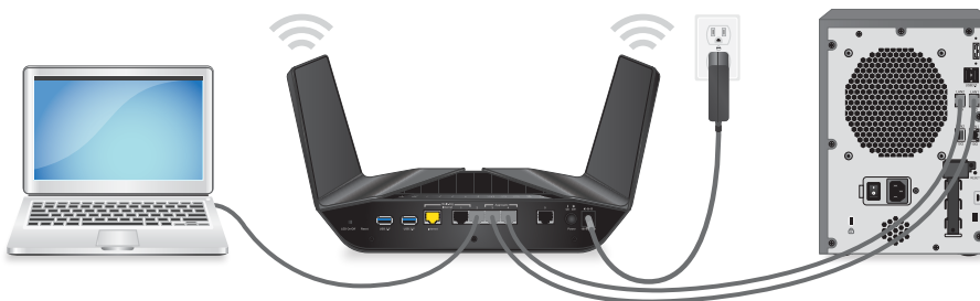
Figure 7. Ethernet port aggregation to a LAN device
